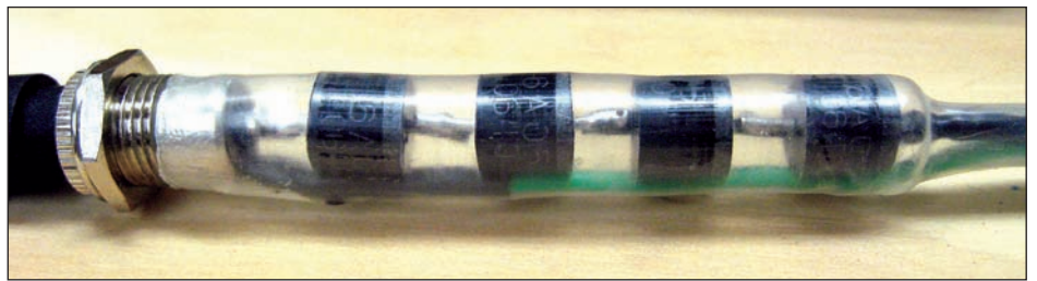
■ FIGURE 7. Four high-current diodes wired in series to drop the 12V power source.
